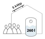
Ex.: If the SMARTFOX System is used only for hot water preparation in a four-person household that requires approx. 2601 of hot water per day, up to 80 % of the required energy can be produced in-house.
