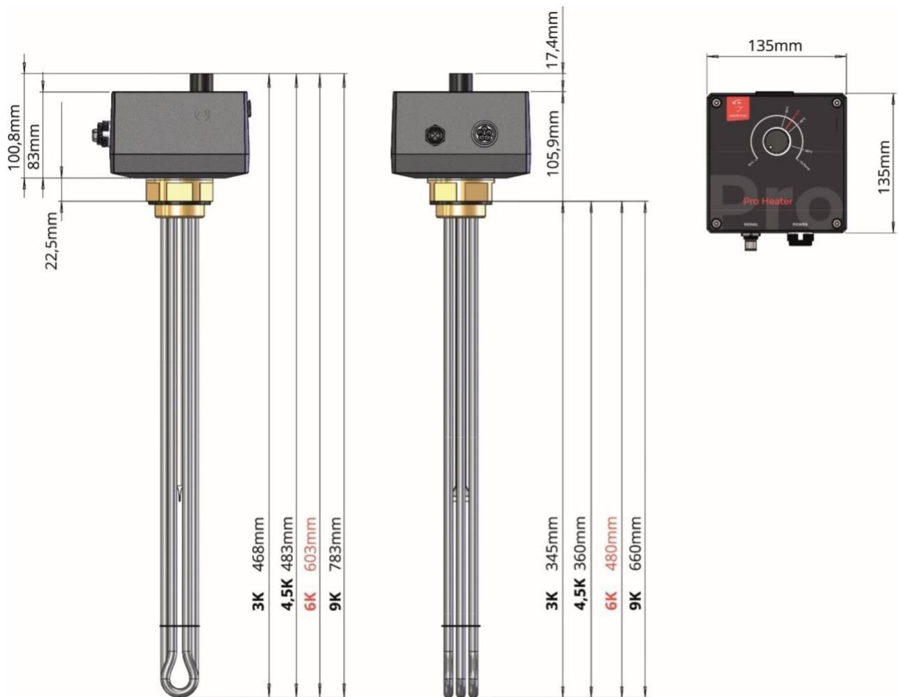
\*The scale refers to the SMARTFOX Pro Heater 6K. The screw-in and total lengths of the product variations are indicated accordingly
